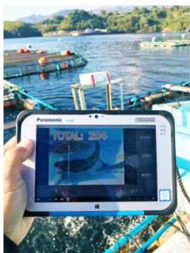
Scene of the automatic live fish counting system in use
