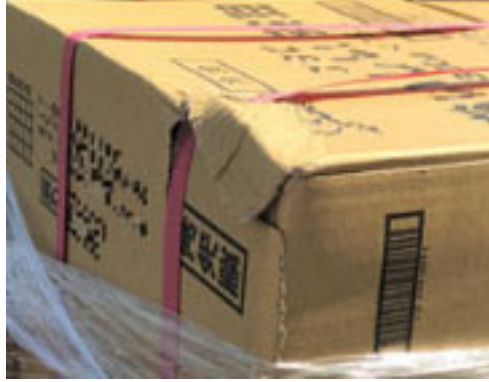
Damage from band penetration
