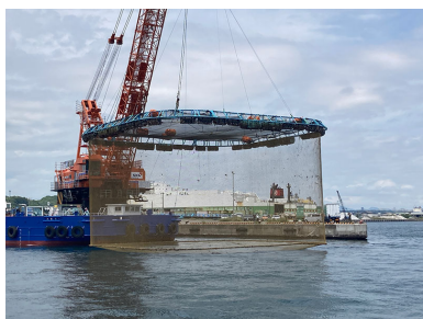
Larger-scale floating and sinking copper-alloy cage with consideration for farming environment.
